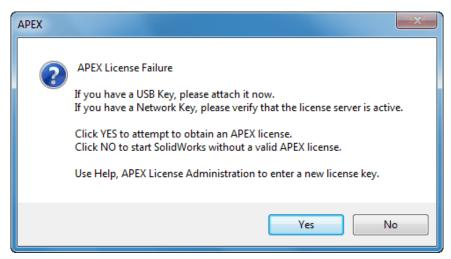
Figure 5 APEX License Failure dialog box - click No to proceed
