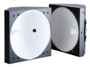
By the barium sulfate coating an average reflection ratio of  $\rho$  = 93% over the visible spectral region. The coating is almost grey and shows a very low change over the wavelength within the visible area.
